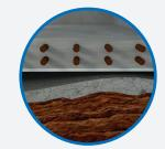
With PREPRUFE®, the membrane is fully sealed to the structural concrete and is unaffected by any ground settlement. The PREPRUFE® membrane remains fully bonded to the structure to resist hydrostatic pressure and avoid membrane stress.
