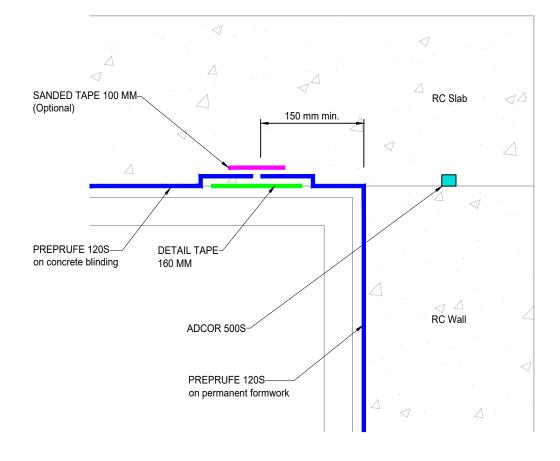
C WALL TO SLAB CONSTRUCTION JOINT Section
